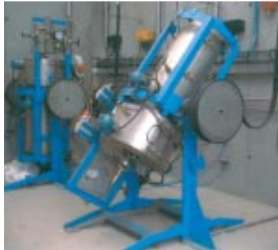
Ageing cells for material samples
