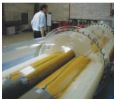
Full-size scale pouring test of bundle gel
